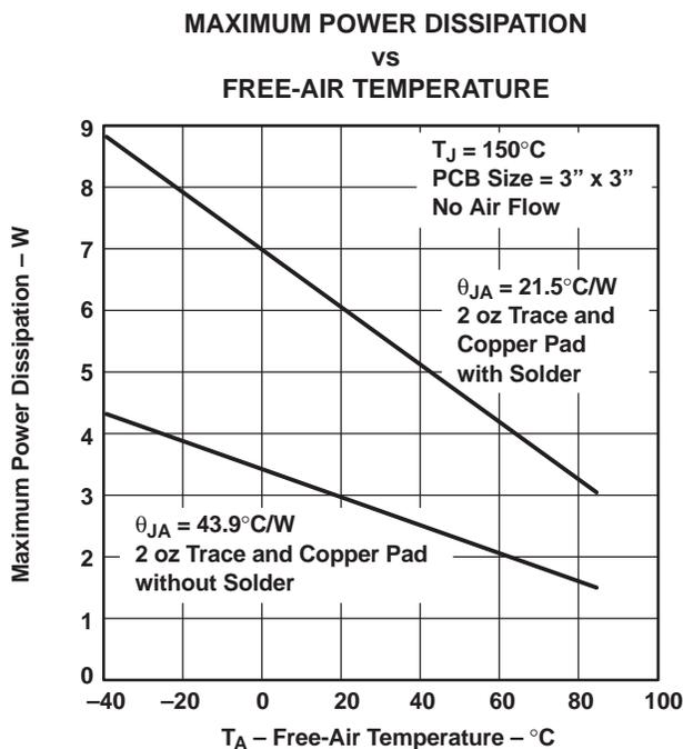
**Figure 46. Maximum Power Dissipation vs Free-Air Temperature**
