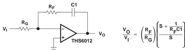
**Figure 50. Inverting CFB Integrator**
