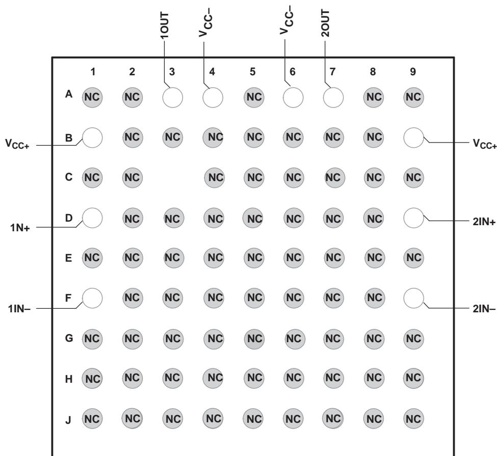
NOTE: Shaded terminals are used for thermal connection to the ground plane.
