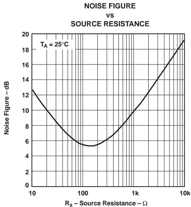
**Figure 42. Noise Figure vs Source Resistance**
