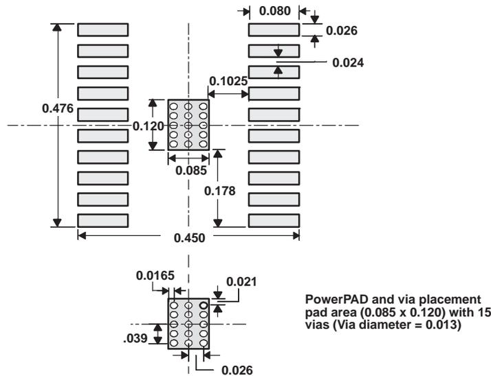
Vias should go through the board connecting the top layer PowerPAD to any and all ground planes. (The larger the ground plane, the larger the area to distribute the heat.) Solder resist should be used on the bottom side ground plane in order to prevent wicking of the solder through the vias during the reflow process.
