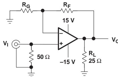
Figure 2. Test Circuit, Gain =  $1 + (R_F/R_G)$
