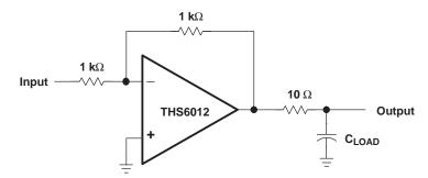
Figure 43. Driving a Capacitive Load
