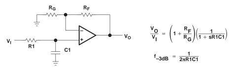
Figure 48. Single-Pole Low-Pass Filter
