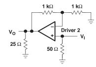
Figure 1. Input-to-Output Crosstalk Test Circuit
