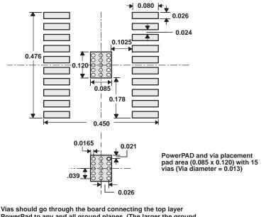
Vias should go through the board connecting the top layer PowerPad to any and all ground planes. (The larger the ground plane, the larger the area to distribute the heat.) Solder resist should be used on the bottom side ground plane in order to prevent wicking of the solder through the vias during the reflow process.
