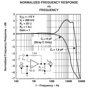
Figure 44. Driver Normalized Frequency Response vs Frequency
