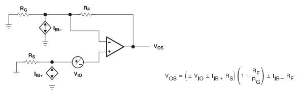
Figure 40. Output Offset Voltage Model
