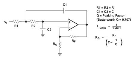
Figure 49. 2-Pole Low-Pass Sallen-Key Filter
